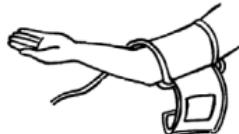
b) Lay the cuff on the arm as illustrated. Make certain that the lower edge of the cuff lies approximately 2 to 3 cm above the elbow and that the rubber tube leaves the cuff on the inner side of the arm.
